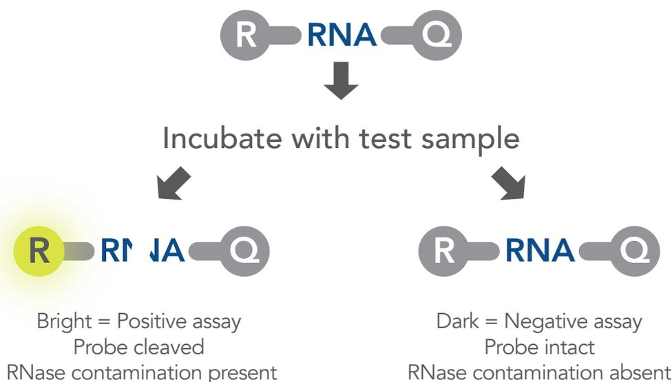
Figure 1. Nuclease detection by RNaseAlert Substrate.
