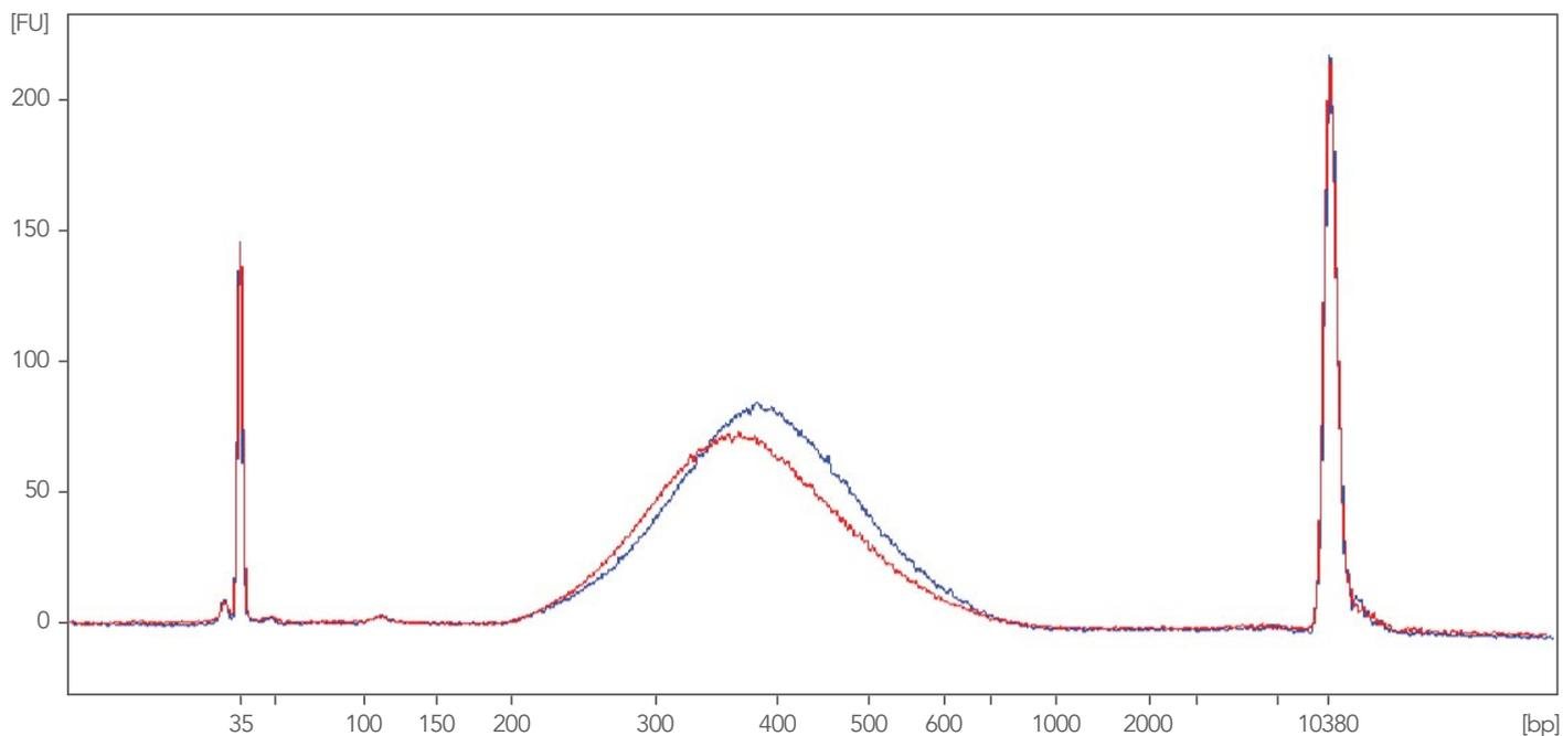
**Figure 5. Bioanalyzer® results for libraries from ribodepleted FFPE RNA.** Expected results for xGen RNA Library Prep Kit libraries produced from 100 ng FFPE RNA following ribodepletion using Lexogen RiboCop v1.3. Libraries were diluted 1:2 and run on the Bioanalyzer using a HS DNA chip.
