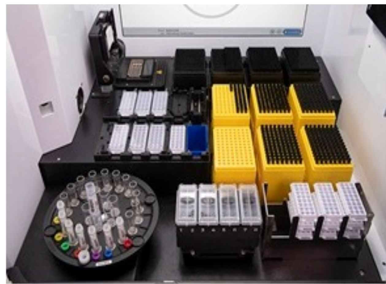
Figure 3. Biomek NGenius Next Generation Library Prep System. Instrument can run 4 to 24 samples. The NGenius Portal can be used for batch setup and remote run monitoring using a customer PC. After batch creation, a work aid is generated for reagent and deck setup.
