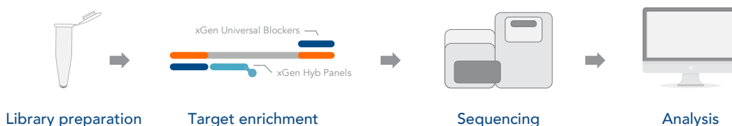
Figure 1. xGen target capture workflow. xGen Universal Blockers bind to adapter sequences during target enrichment using xGen Hyb Panels.
