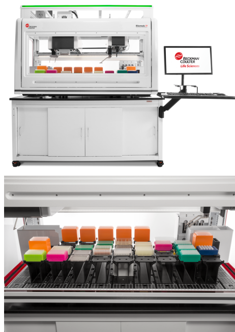
Figure 1. Biomek i7 Hybrid Genomics Workstation with optional Enclosure on a Biomek Mobile Workstation. Deck layout in the lower image.
