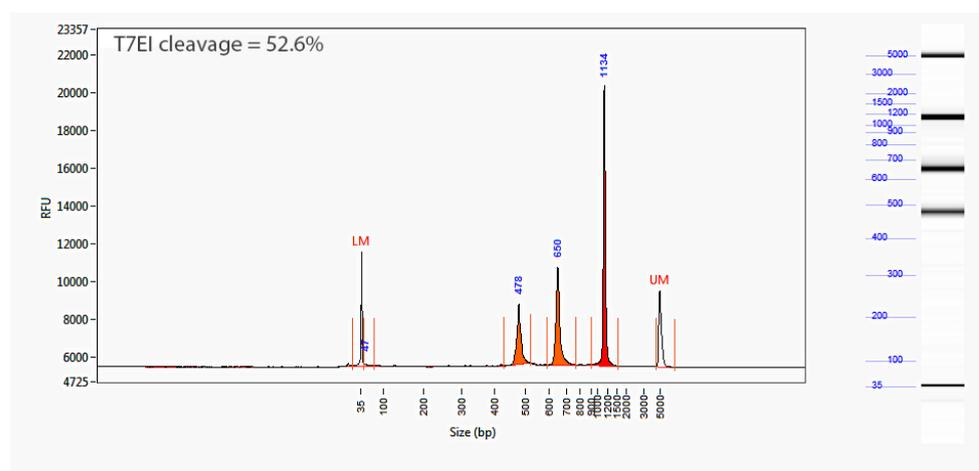
**Figure 4. Representative results of a digestion from a Fragment Analyzer™ system.** Percent cleavage = Average molar concentration of the cut products / (Average molar concentration of the cut products + Molar concentration of the uncut band) × 100. LM = lower marker; UM = upper marker.
